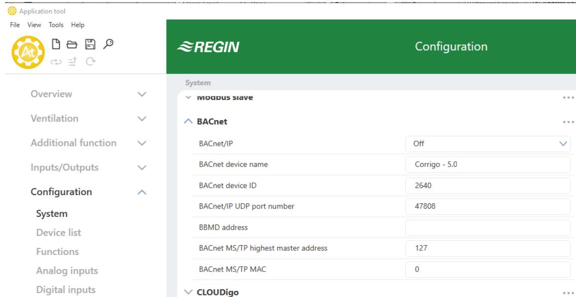
Figure I-1 BACnet configuration in Application tool
