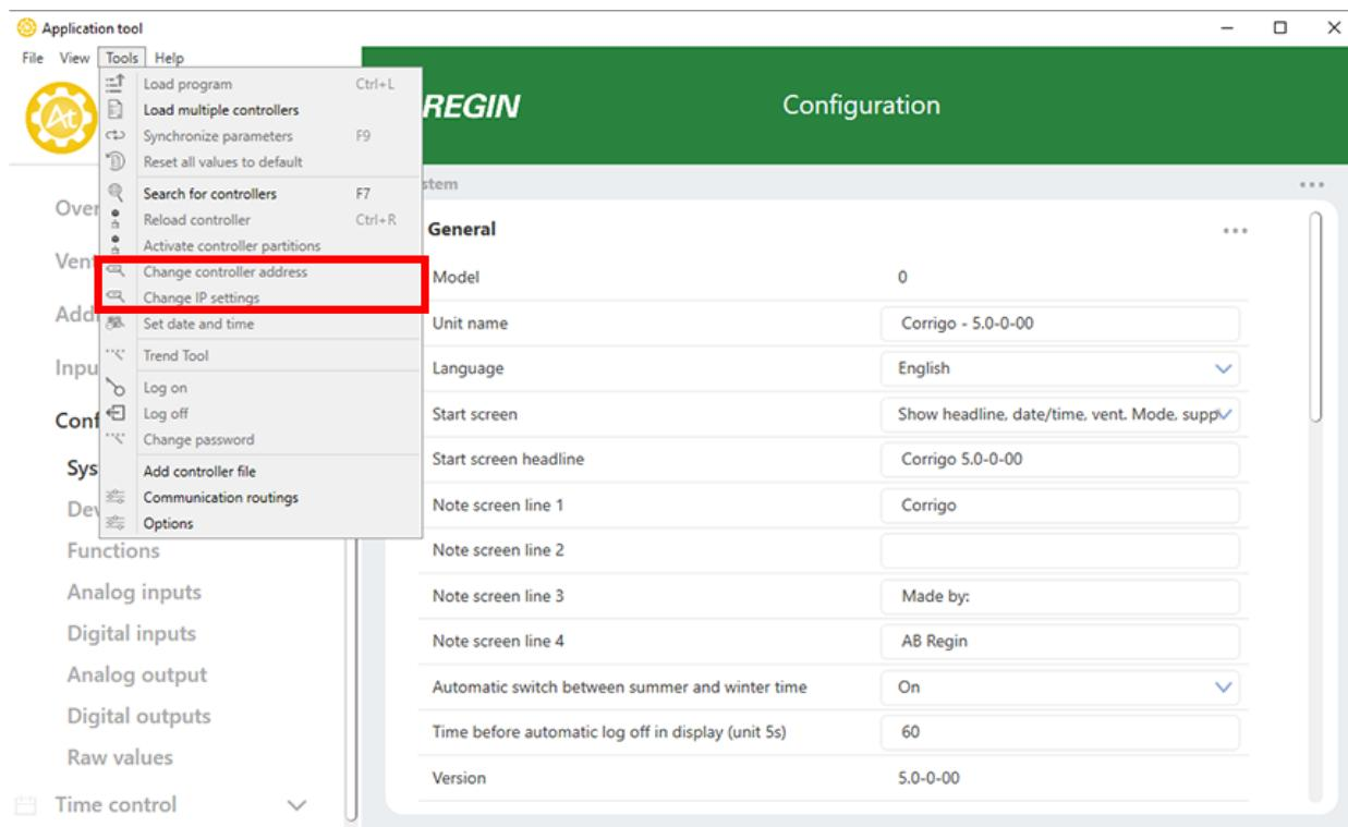
*Figure 1-2 Changing the controller address and IP settings*
