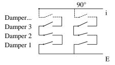
When the test cycle is initiated, the output "Fire dampers" will be activated and the dampers will begin to move. Within the set time (90 sec) the signal on "Fire damper end-switch monitoring" must change to indicate that the dampers have left their normal positions. If not an alarm will be triggered.
