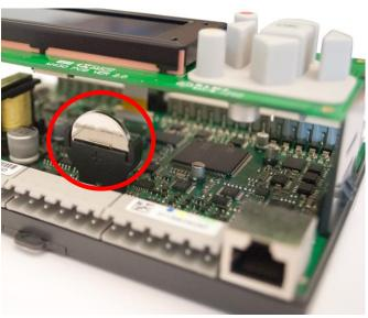
Grip the battery firmly with your fingers and lift it upwards until it rises from its holder.
