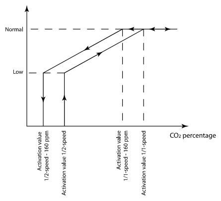
When used with 2-speed fans they will start using reduced speed when the  $CO_2$  value rises above control value one and switch to normal speed when the  $CO_2$  value reaches control value two. The fans will stop when the  $CO_2$  value falls 160 ppm below control value one.
