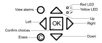
There are seven buttons: four arrow buttons which will be called UP, DOWN, RIGHT and LEFT. The menus in the Corrigo are organized in a horizontal tree structure. The UP/DOWN buttons are used to move between menus at the present menu level. The RIGHT/LEFT buttons are used to move between menu levels. When changing parameters the UP/DOWN buttons are used to increase/decrease the value of the parameter and the RIGHT/LEFT buttons to move between digits within the parameter.
