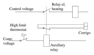
Wiring suggestion high temp limit when using electric heating.
